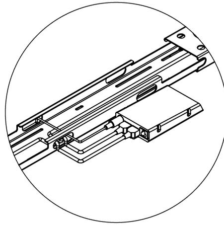
9. Connect all cables to the control box in the correct connectors
