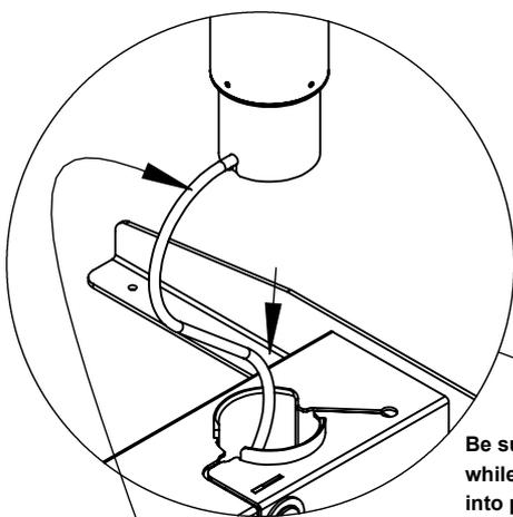
Be sure to pull the cord, while inserting the column into position
