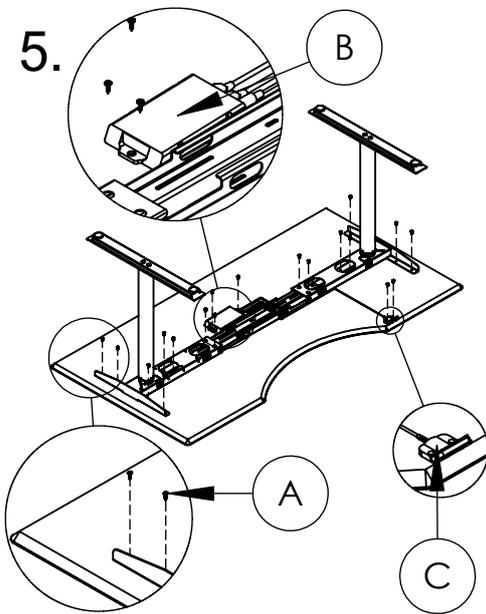
8. Screw the frame, control box and hand control to the desk
