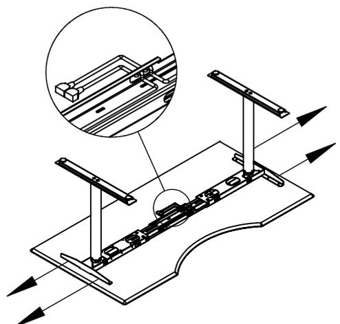
7. Pull the SIDE FRAMES away from the MIDDLE PIECE, and move the column wires out through the hole in the MIDDLE PIECE
